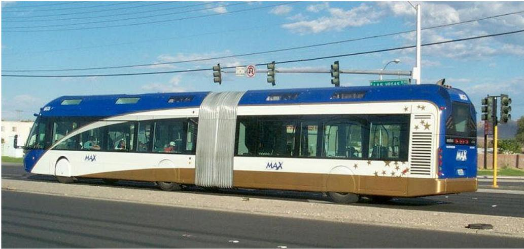
**Figure 3.** Civis diesel-electric hybrid bus
