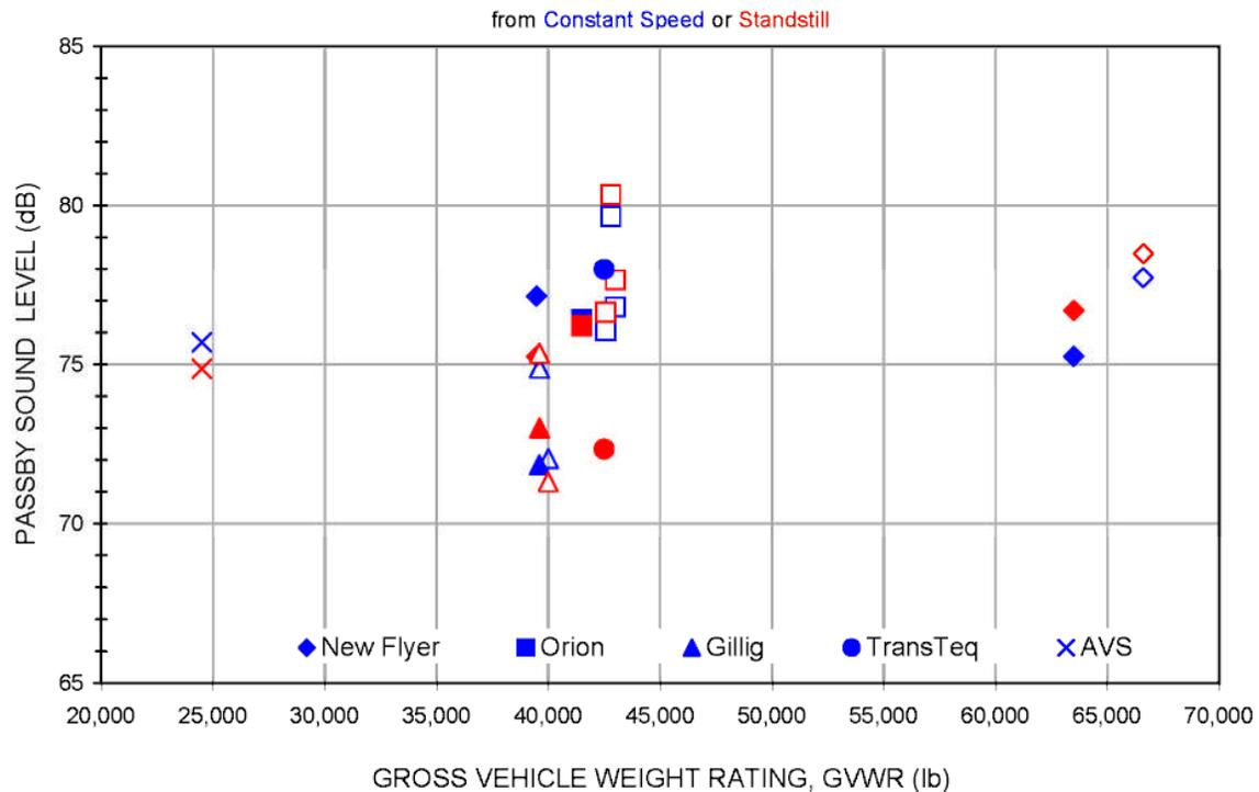
**Figure 1.** Conventional v. Hybrid Bus—Accelerating Pass-By Sound Levels
